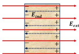
Metal Body An electrical field gets develop inside the metal due to induced charges.
